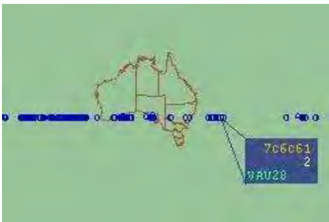
Figure 1 - Track Jumping problem with TPR901
